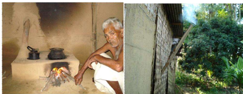
Udairaj chullah in use in one of the household with the inclined chimney pipe through the sidewall
